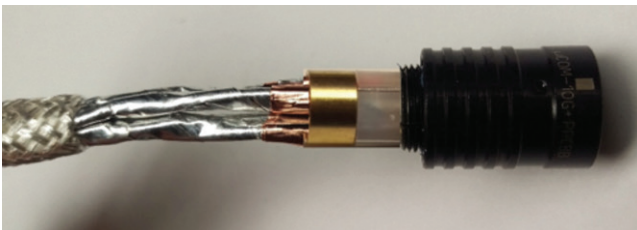
Figure 24: Seating the crossbar washer
