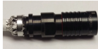
Figure 47: Trimming excess braid on plug
