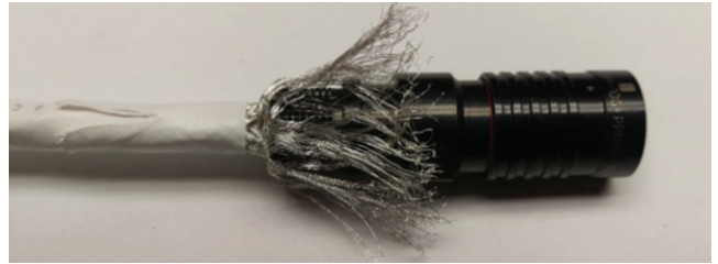
Figure 27: Brushing the braid
