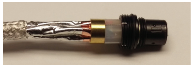
Figure 41: Seating the crossbar washer
