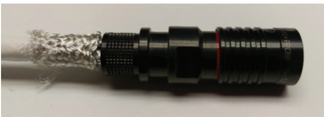
Figure 26: Returning the braid
