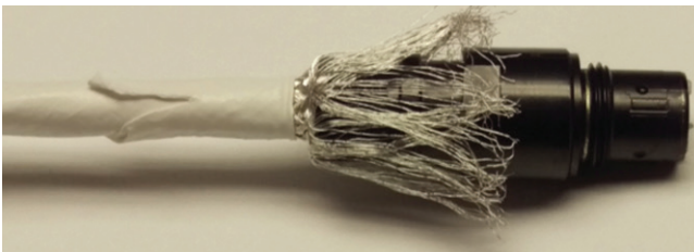
Figure 44: Brushing the braid
