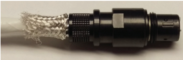
Figure 43: Returning the braid
