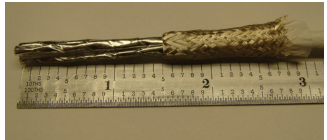
Figure 15: Exposing the foil
