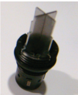
Figure 37: Replacing the crossbar
