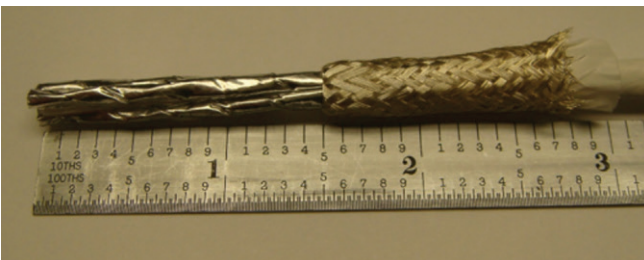
Figure 32: Exposing the foil
