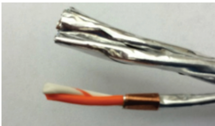
Figure 18: Removing the foil edge
