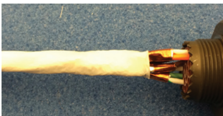
Figure 43: Returning the outer jacket
