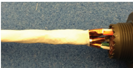
Figure 27: Returning the outer jacket
