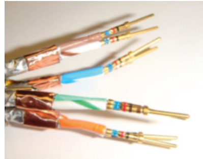
Figure 38: Stripping and crimping the contacts
