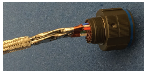
Figure 22: Inserting contacts into connector
