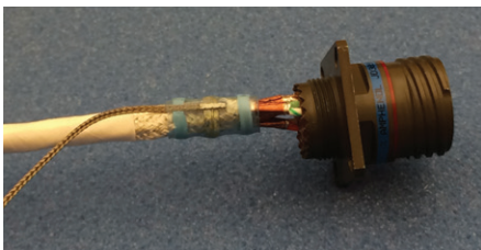
Figure 42: Sliding the solder sleeve ground lead (S200-5-01)
