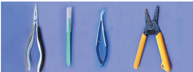
Figure 1: Needle nose pliers, scalpel, tweezer scissors, and hand strippers
