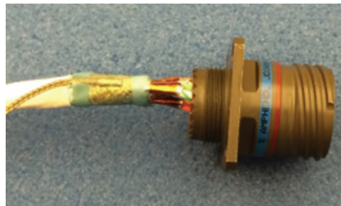
Figure 45: Returning the outer jacket
