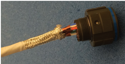
Figure 24: Sliding the braid back
