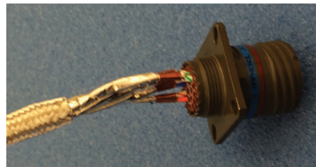
Figure 39: Inserting contacts into connector
