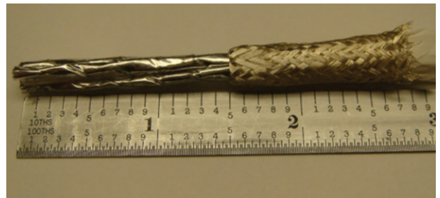
Figure 15: Exposing the foil
