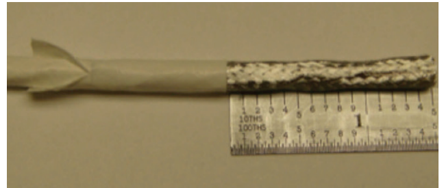
Figure 31: Exposing the braid
