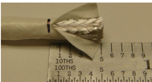
Figure 30: Slitting the cable jacket
