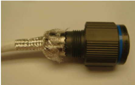
Figure 23: Folding the braid over the backshell
