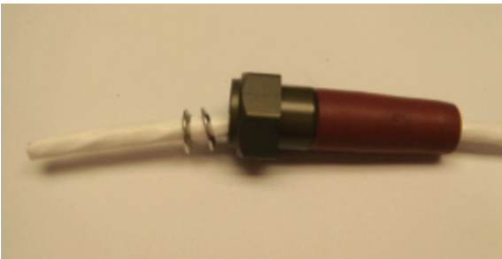
Figure 11: Sliding the backshell onto the cable
