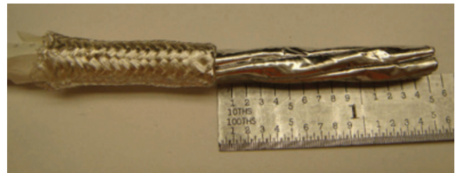
Figure 32: Exposing the foil
