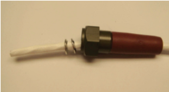
Figure 28: Sliding the backshell onto the cable
