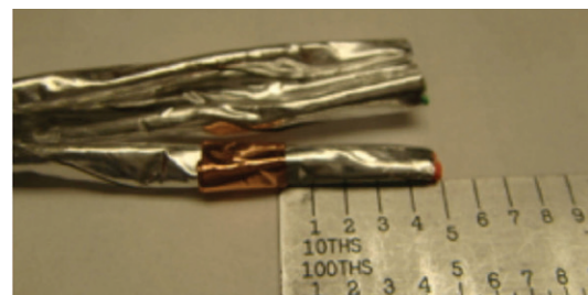
Figure 16: Wrapping the foil
