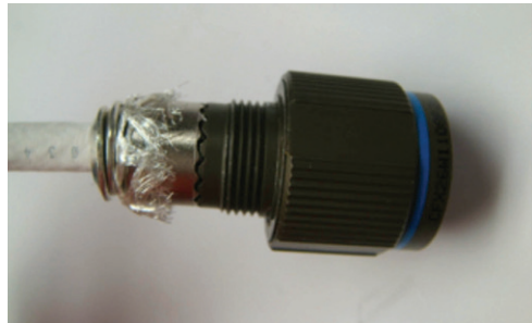
Figure 26: Placing the washers near the connector
