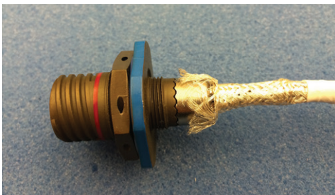
Figure 40: Folding the braid over the backshell
