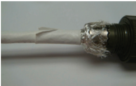
Figure 24: Returning the jacket to the connector
