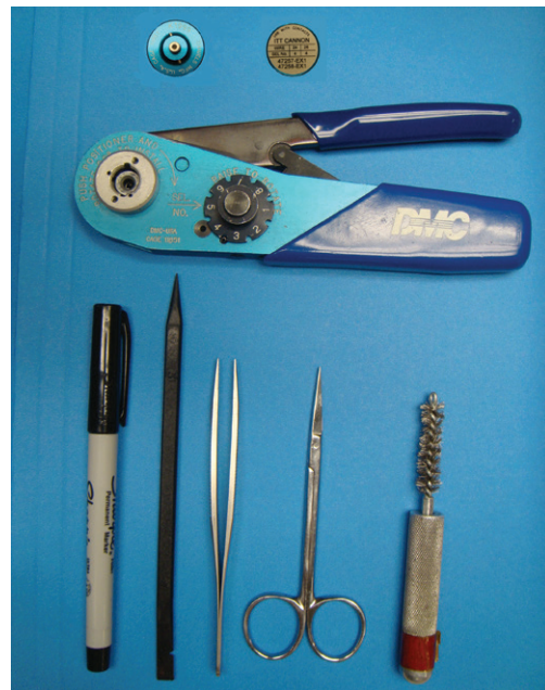
Figure 4: ITT Cannon Crimp Die, DCM Crimper (M22520/2-01), Sharpie, plastic pick, tweezers, small scissors, and braid brush
