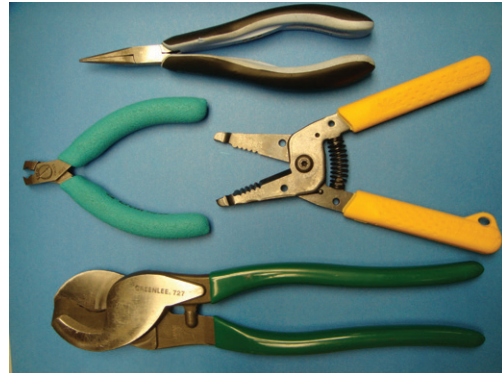
Figure 3: Soft-jawed pliers, flush cutters, hand strippers, and round cable cutters
