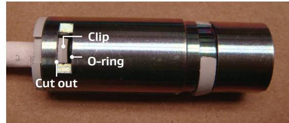
Figure 82: Lining up the clips with cutouts
