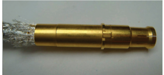
Figure 31: Installing outer body
