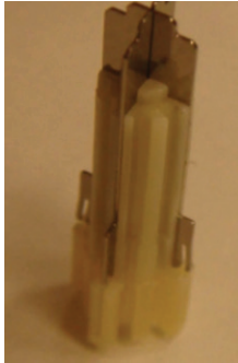
Figure 46: Inner insulator with metal spacers
