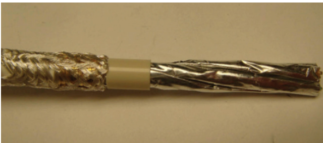
Figure 17: Sliding plastic bushing onto cable
