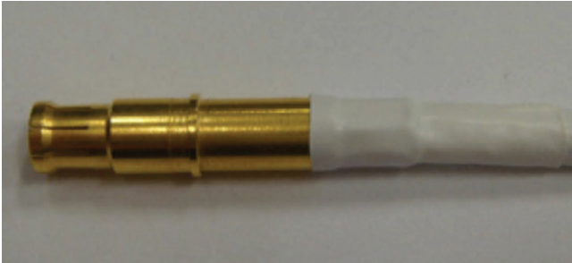
Figure 62: Shrinking tubing on crimp socket
