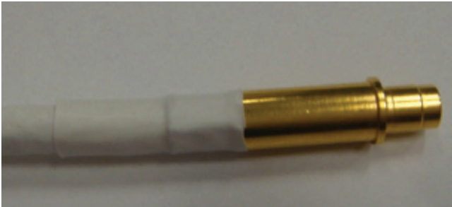
Figure 63: Shrinking tubing on crimp pin
