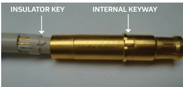
Figure 30: Aligning the keyway
