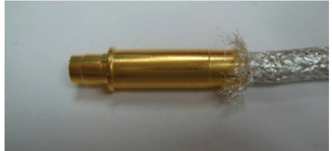
Figure 55: Installing outer body
