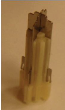
Figure 22: Inner insulator with metal spacers
