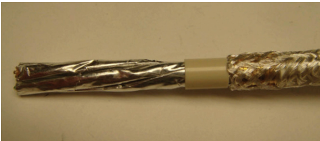
Figure 41: Sliding plastic bushing onto cable
